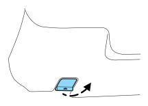
2. Go to the front of the vehicle and release the auxiliary latch using the handle that is located under the front passenger side of the hood.
